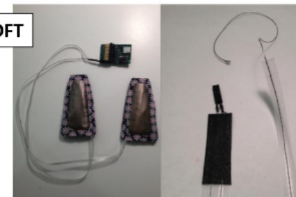
Straight Dipole 2.7 dBi
